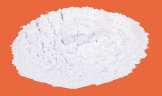
Castable Refractories are dry, granular refractory mixtures designed to be mixed on site with water and are capable of curing to a stable dimensional form through hydraulic or chemical setting. They can be used for molding complete furnace linings and other unique shapes at installation sites. Asfour M&R can supply a full line of refractory castables utilizing various bonding systems.
